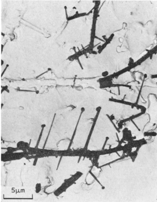
Figure 13 Side growths after 17 h at 1100°C in argon.
