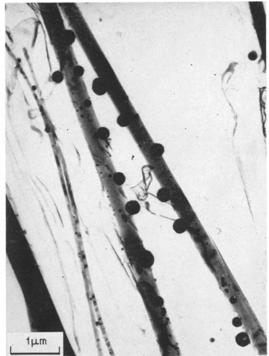
Figure 6 Nickel coated whiskers after 30 min at 1000°C in vacuum.
