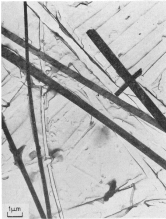
Figure 1 Silicon nitride whiskers after 17 h at 1100°C in vacuum.
